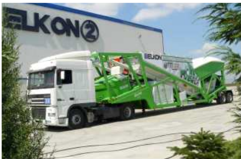
The Elkon Mobile Master -60 concrete batching plant is fully mobile
