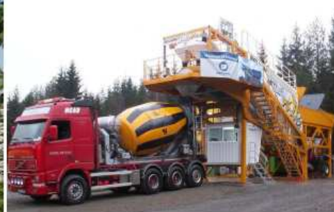
The working position of the mobile concrete batching plant
